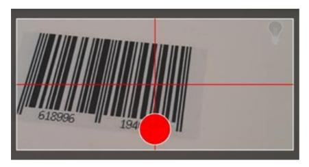
The viewfinder in the above image has an active scanning surface, a result of having set active symbologies. For more details on this topic, see <u>Configuring the Reader Device</u>).
