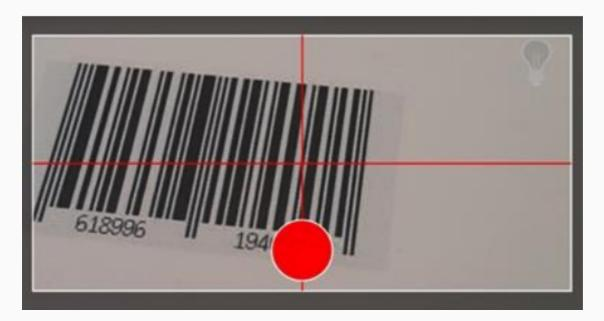
The viewfinder in the above image has an active scanning surface, a result of having set active symbologies. For more details on this topic, see <u>Configuring the Reader Device</u>).
